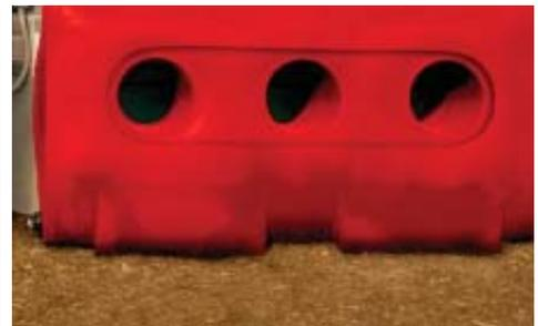
9. Position the tank leaving at least 3 inches of space from the wall. Be aware that the spigot goes on the bulkhead that is attached to the pump and flexible hose. Check for clearance on all sides and be sure the tank is not creating an obstruction for anything else.
