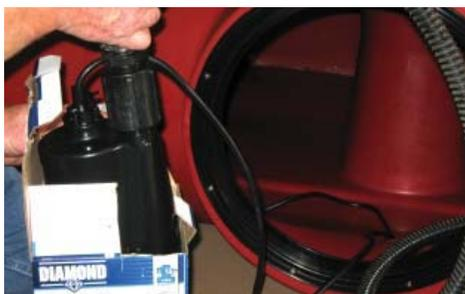
2. Remove the submersible pump in the tank by pulling the flexible hose. Take the pump out of its cardboard box and hold on to any documentation for later reference.
