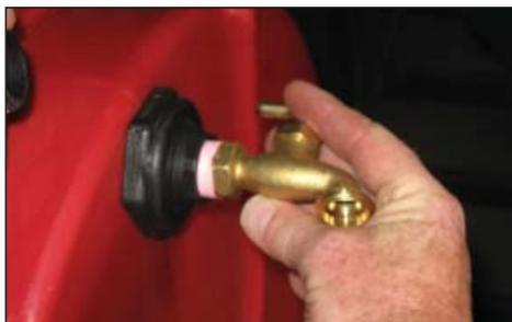
11. Attach the spigot to the bulkhead connected to the pump inside the tank and hand tighten. Using an adjustable wrench, tighten the spigot another full rotation after hand tightening.
